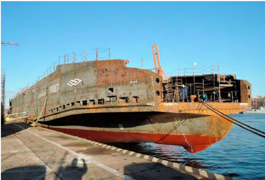
The hull of *Piret* shortly after launching and tow-out.
