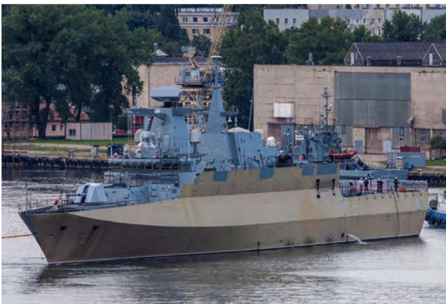
On July 28 the ship TBN ORP *Ślązak* was towed from inside of the yard to Nabrzeże Gościnne pier of Naval Shipyard Gdynia. The aim was to carry out drives and propulsion system tests, including main propulsion stationary tests.
