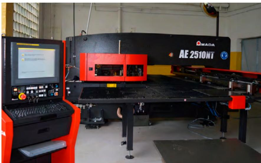
Famor enhanced its production machinery portfolio with an AMADA make AE-NT punching machine offering a punching capacity of 200 kN, with working area of 2500 by 1270 mm without repositioning and plates thickness up to 3 mm. It provides high precision (0.1 mm accuracy), numerically controlled steel and alloy plates punching.
