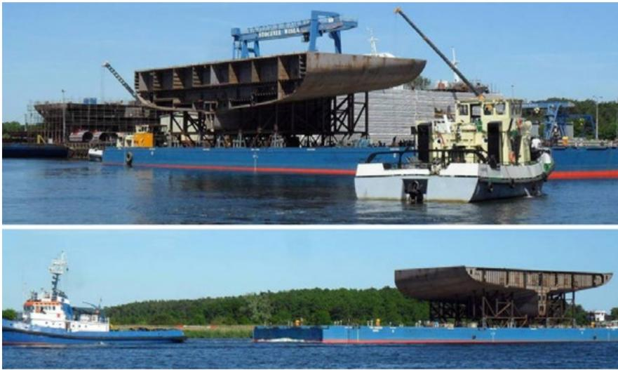
On June 7, 2018, another shipment left the Wisła Shipyard - a bottom block of the aft part of a cruise ship with a part of a stern skeg, loaded on the *TRD Horizon* pontoon-barge (80 × 25 m). It was the first shipment this yard to Meyer Turku in Finland.
