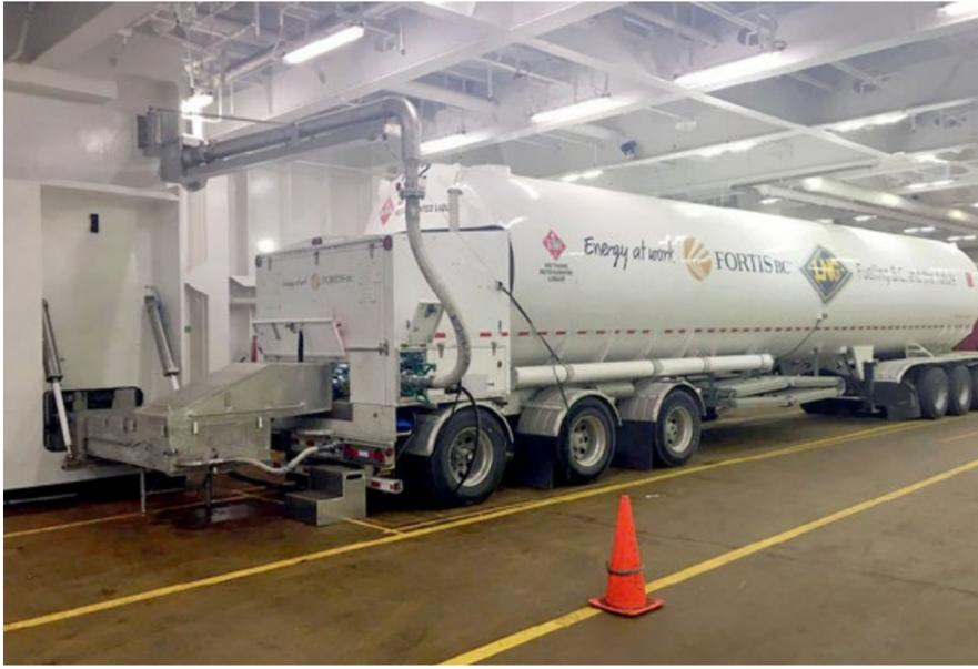
LNG road tanker at bunkering station on an enclosed car deck of the *Spirit of British Columbia* ferry.
