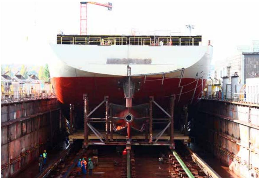
The hull of the B 204/1 unit while being rolled onto a dock.
